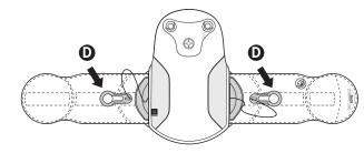
Lay brace on a flat surface then pull both Wings outward to reset the tightening mechanism
