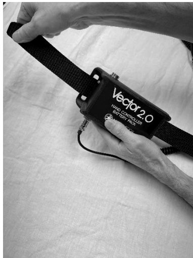
Thread belt through the battery pack.
