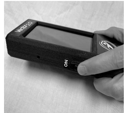
Slide the toggle switch to the "on" position.
