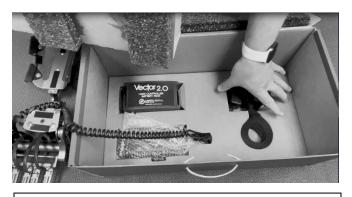
The (2) strips of foam padding should be rest over the nylon belt and (2) wall power adapters.
