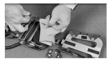
Remove and discard the Vector 2 glove by detaching glove away from the finger shoes.
