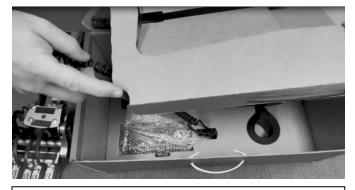
Note: The corner of the Upper Tray will have a small cutout. This is where to route the LCD hand controller cable from the Lower Tray to Upper Tray.
