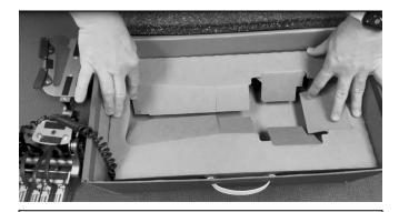
Insert the Upper Tray, as shown. Note: The cable routing from Lower Tray. The Vector 2 Box handle will rest inside the middle of the Lower Tray.
