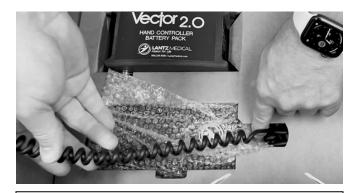
Insert the LCD hand controller, as shown. Tuck the open-ended cable inside the middle of the Lower Tray. If possible, use the original LCD bubble wrap.
