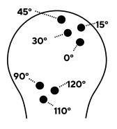
The flexion and extension stops on Townsend Low Profile ROM elbow braces can be adjusted using the flathead screws provided with the brace. The screws are preset in the 0 degree extension stop hole and 90 degree flexion stop hole. Only a small flathead screwdriver is required to remove the screws.
