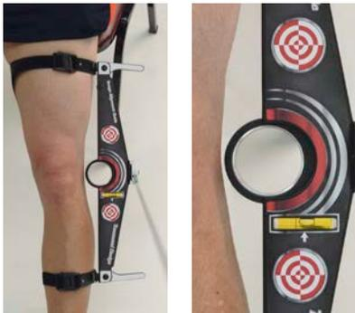
**Step 7:** Take a picture. Look at the image to confirm: 1) no toe out; 2) the bubble is in the center of the level; and 3) the image only shows the SILVER RIM of the Focal Angle Tube and not the red inside walls. We suggest you take and submit 2-3 front view pictures -- so we can choose the best image.
