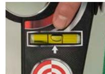
**c)** Adjust the tilt of the IAG until the bubble is centered (or not touching either end) of the level tube.
