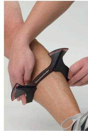
**Step 10:** Apply the Tibial Contour Gauge (6, 7 or 8 inches below the patella) and center the gauge on the crest of the tibia. Move/adjust the two alignment arms until the device is in full contact with the medial and lateral contour of the shin with no gapping.
